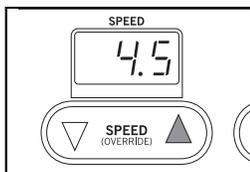
As you exercise, change the speed of the walking belt as desired by pressing the SPEED buttons. Each time one of the buttons is pressed, the speed will change by 0.1 mph. If the buttons are held down, the speed will change in increments of 0.5 mph. The speed range is 0.5 mph to 10.0 mph.
