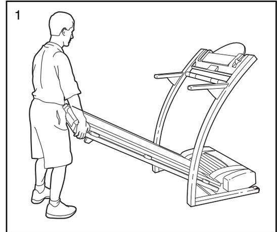
2. Move your right hand to the position shown and hold the treadmill firmly. Using your left hand, pull the latch knob to the left and hold it. Raise the treadmill until the latch pin is aligned with the hole in the catch. Insert the latch pin into the catch. **Make sure that the latch pin is fully inserted into the catch.**
