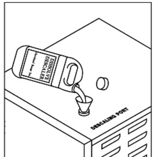
Figure 6-1 Descaling Port Located at Right Rear of the Combi
