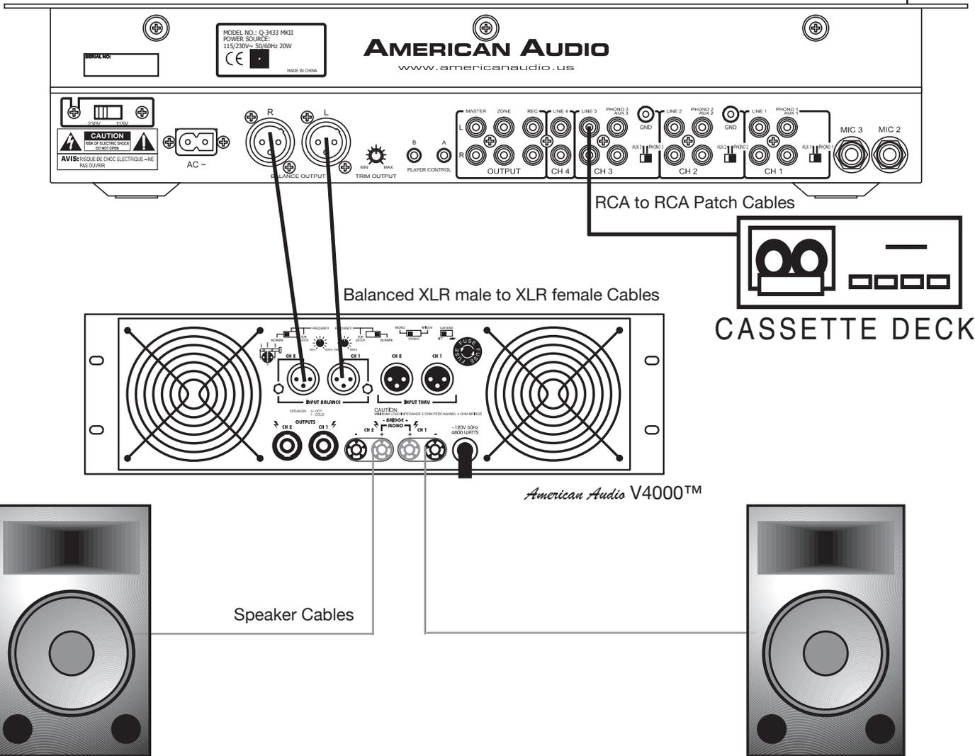
**Typical Balanced Output Set-up**
