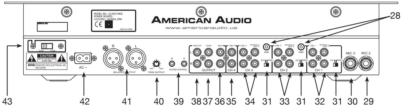
**28. GND (GROUND TERMINAL)** - Be sure to connect turntable ground leads to either or both of the two available ground terminals. This will reduce the humming and popping noises associated with magnetic phono cartridges.
