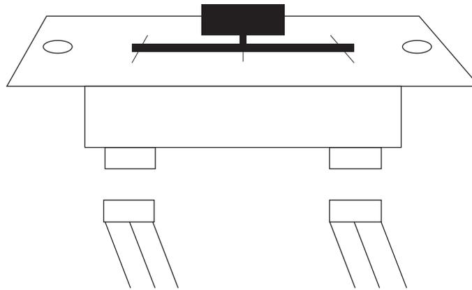
The crossfader is “Hot Swapable” which means it may be replaced at any time, even when power is applied. Only replace with American Audio Part Feather Fader Plus. Replacing with any other model fader may seriously damage your mixer.
