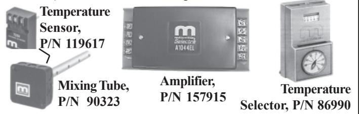
Option AG36 is a special application gas train that is designed for controlling the environment of a paint booth operation. The system includes a Maxitrol A1494 amplifier, discharge air temperature sensor, dual remote discharge air temperature selector (drying selector 80-140°F and a spray selector 60-90°F), and two switches to control the operation of the modulating gas valve.
