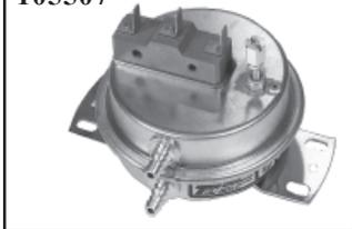
switch is only on systems with an optional console that includes a dirty filter light. The pressure switch is set during installation so that the light will be activated at approximately 50% filter blockage. Contacts should close at .17 to 5.0" w.c.  $\pm$  .05" w.c.
