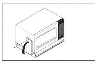
Assemble the **Bracket Left** to outer panel.
