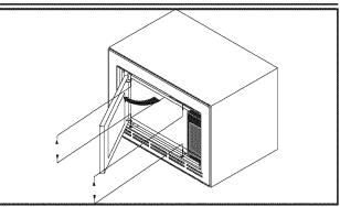
Fix 2 screws each at the upper and lower parts of **Trim Frmae** with the door open.
