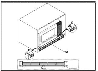
Place **Bracket Bottom** on **Bracket Base** like picture **B**. Make holes of position **A** fit to **Bracket Base**'s and fix screws after making holes with a 7/64 drill or a #35 drill.
