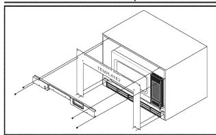
With template 2, make 2 holes each at the upper right and left parts of cabinet. (Others for the extra) Fix "Bracket Top" according to the holes.
