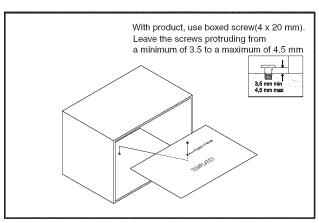
Fix '1" screw' at the bottom of cabinet with use of template 1.
