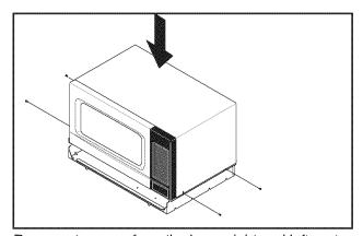
Remove 4 screws from the lower right and left parts of outer panel, place "SET" in **Bracket Base** and fix it by tightening 4 screws again.
