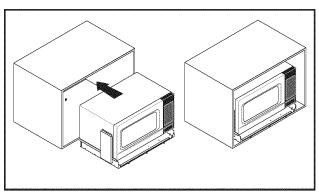
Push "SET" into the cabinet inside so that the fixed bottom screw of cabinet can place in the hole of Bracket Bottom.
