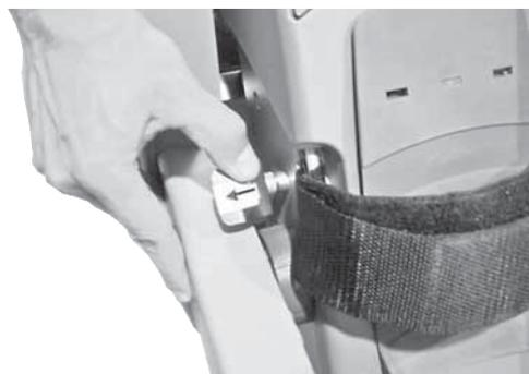
3. Lower the front frame carefully in between the rails and lock it with the retainer in the front end of the seat. Ensure that the front frame is locked.
