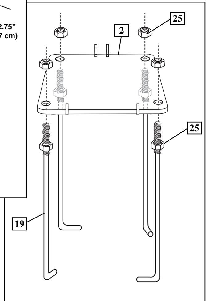
3. Install threaded ends of J-bolts (19) through holes in mounting plate (2) and secure as shown.
