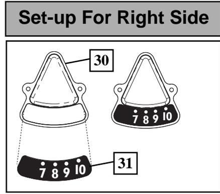
B. Attach height indicators to lower yoke in area shown by turning screws (29) into place with a phillips-head screwdriver. Apply name plate sticker (15) to lower yoke as shown.
