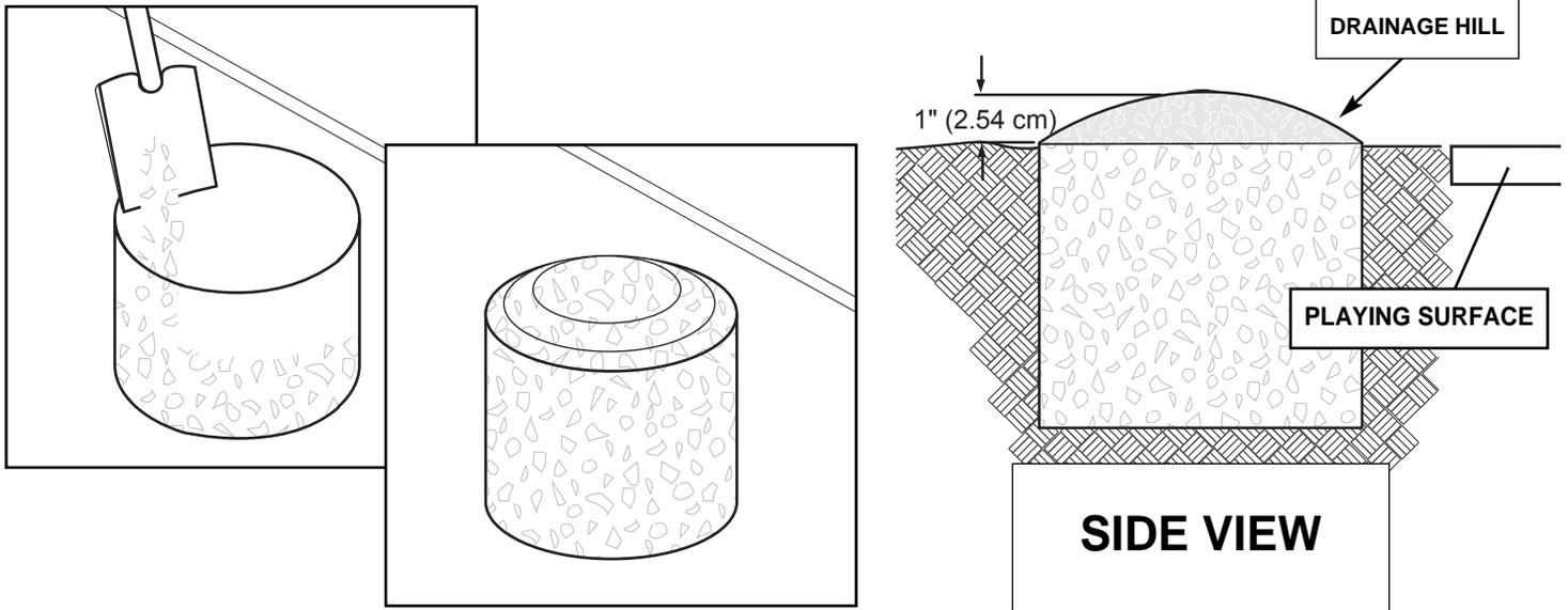
5. Insert J-bolts (19) from mounting plate (2) into cement as shown. Move assembly around to release any air pockets in cement, then rest mounting plate on cement drainage hill. Apply some pressure to level mounting plate on top of drainage hill. Level mounting plate and square with playing surface. Clean off any excess cement on mounting plate at this time and place washers (24) on J-bolts (19).
