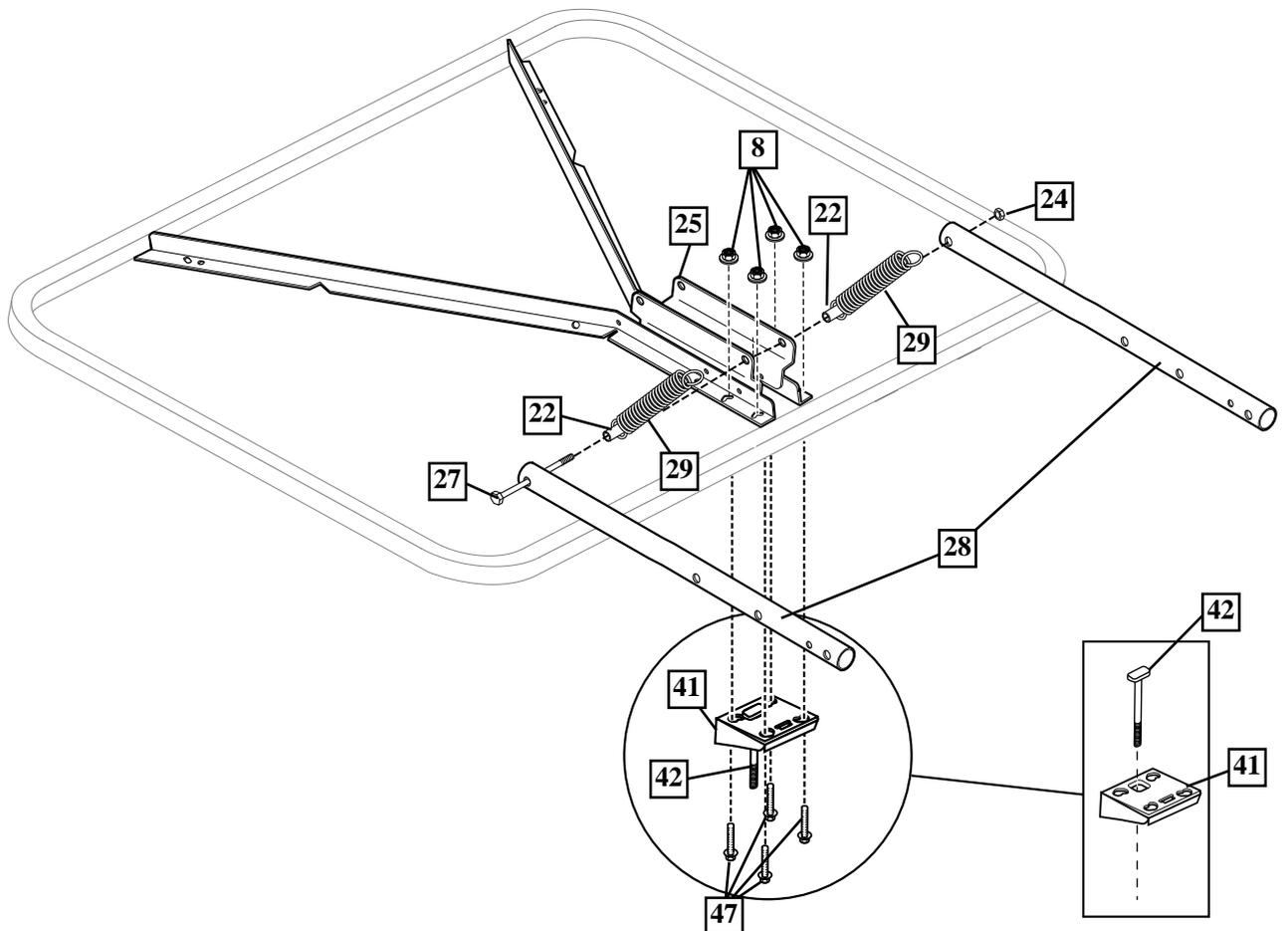
**3.** Attach upper elevator tubes (30) to backboard support brackets (25) using spacers (22), bolt (27), and nut (24) as shown.
