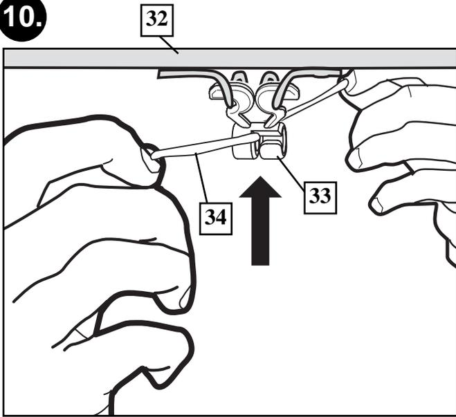
Insert net into bottom of clip as shown.
