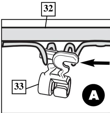
Insert one "arm" of clip into ram as shown. Twist "body" of clip slightly so that second "arm" slides over the top of the first "arm" as shown. Push in direction indicated by arrows.
