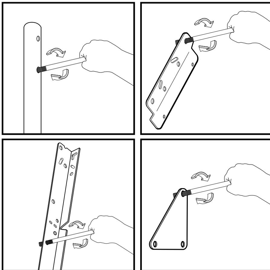
**To ensure optimal playability of backboard system, a close tolerance fit between the elevator components and hardware is required. Test fit large bolts into large holes of elevator tubes, backboard brackets and triangle plates. Carefully rock them in a circular motion to ream out any excess paint from holes if necessary.**
