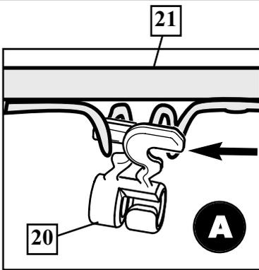
Insert one "arm" of clip into ram as shown. Twist "body" of clip slightly so that second "arm" slides over the top of the first "arm" as shown. Push in direction indicated by arrows.
