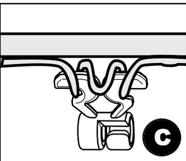
Twist "body" of clip slightly again to spread "arms" of clip. Clip "arms" must be flat and touching edge to edge as shown, not overlapping.
