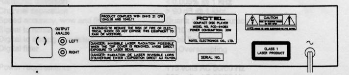
Please refer to this drawing of the Rear panel of the RCD 940BX when connecting to your stereo system.
