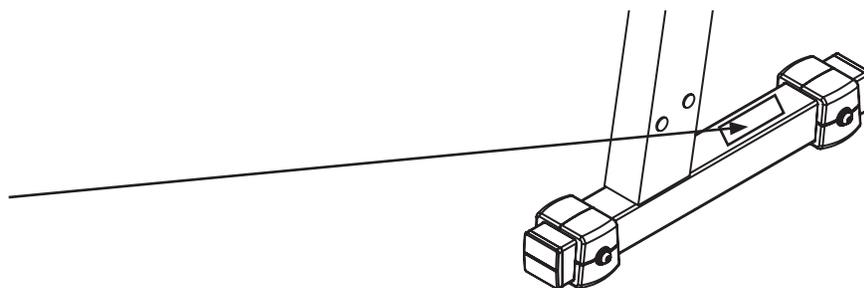
**NOTE: Hand tighten bolts and nylon nuts until machine is fully assembled.**
