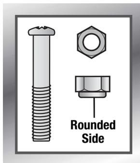
**Tip:** If you cannot attach the M5 lock nut to the end of the M5 x 29 mm bolt, you have assembled the crossbar incorrectly to the L tubes. Turn the crossbar around. Make sure the white dot on the crossbar matches the white dot on one of the L tubes.
