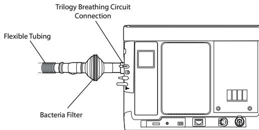
2. Connect the other end of the flexible tubing to a separate exhalation device.
