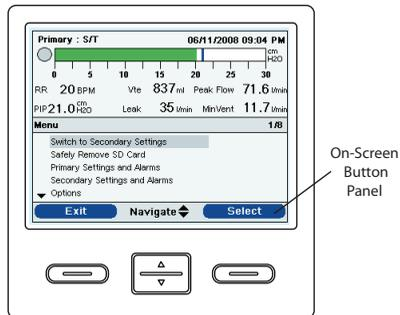
At the very bottom of the display screen is the on-screen button panel. This panel corresponds with the control buttons on the ventilator:
