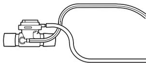
1. Connect the flexible tubing to an active exhalation device with proximal pressure.
