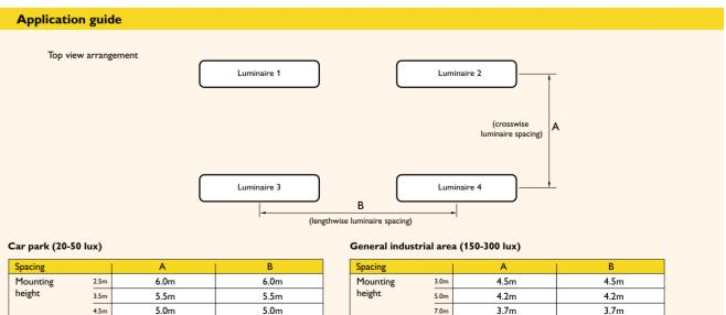
Note: Lighting level >=150 lux with 2x28W and 2x36W, >=200 lux with 2x35W and 2x58W
