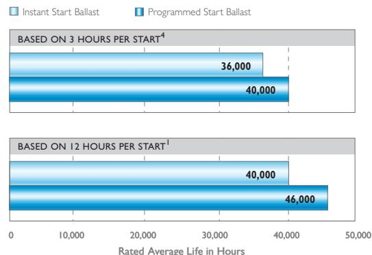
4) Average life under specified test conditions with lamps turned off and restarted no more frequently than once every 3 operating hours. Lamp life is appreciably longer if lamps are started less frequently.
