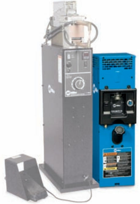
Coolmate V3 shown with stationary spot welder
