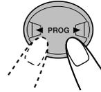
Each time you press the button, the tape direction changes alternately.
