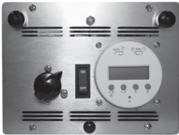
Item 1: Ventilation Timer & Humidity Control
