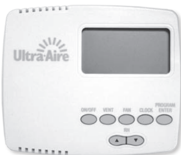
Item 3: DEH 3000 Digital Control
