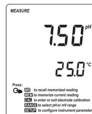
In order to take more accurate pH measurements, make sure that the instrument is calibrated (see page 9 for details).
