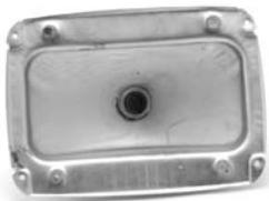
5. Loosen the lens seal from the housing by gently pulling the seal away from the housing.
