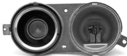
7. Feed the wires through the larger hole in the mounting plate. Guide the mounting plate to the bottom of the housing. The flat side of the mounting plate should be down and the side with the slight raised center should go up into the housing. This will align the mount in the original housing.
