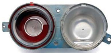
3. Now is a good time to clean the lens and housing. If lenses are in bad shape a new set is recommended.
