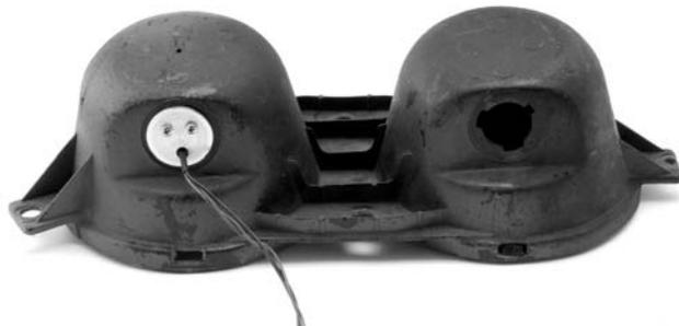
10. Install the lens and/or re-assemble the tail light housing, insuring all gaskets are intact and in place. Install the tail light housing back into the vehicle. You are now ready to wire the LED assembly into the vehicle tail light harness.
