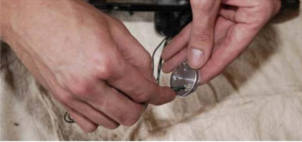
8. Now hold the LED assembly so that it is centered over the hole where the original bulb was located and align the mounting plate from the bottom with the slot in the housing. The screw holes should be lined up.
