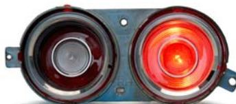
1. Remove the tail light assembly from the vehicle by removing the original bulb sockets from the housing. Then remove the housing hardware so it can be removed from the car. Remove the housings from the vehicle carefully so the housing to body gaskets are not damaged.
