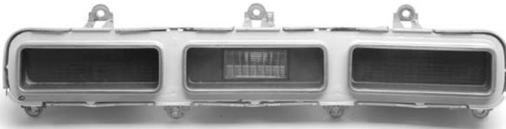
10. Cut off the existing light socket as it will not be used. Do not strip the wires. Trim the wires from LED assembly to appropriate length once mounted, making sure wires are routed cleanly and securely.
