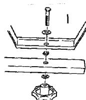
**Step 3:** To attach the light assembly bar to the adjustable pole, position the hole in the middle of the light assembly bar over the threaded screw on the pole. **NOTE:** The large hole in the light assembly bar should be facing down to fit over the nut already in place. Once the light assembly bar is in place, position the hole in the Y-connector over the threaded screw. Secure with attachment knob (J).
