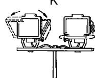
**Step 3:** Adjust the tripod stand to the desired height by loosening and tightening the locking collars on the pole (L).
