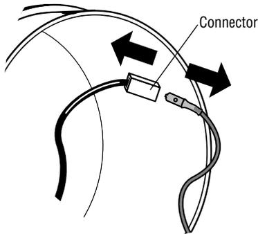
**Step 9:** Reconnect the bulb wire to the connector.
