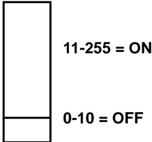
**If the value of channel A is set between 0 to 10, the unit is off.**
