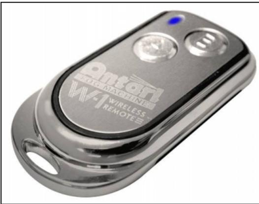
With the transmitter it is possible to emit fog via radio over a distance of up to 50 meters. The transmitter is compatible to any receiver of HZ-350 and can control an unlimited number of machines in parallel. Press the button “**A**”, to emit fog. As control, the LED on the transmitter is lit. To stop the fog output, press the button “**B**”.
