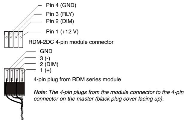
FIG. 2 Connecting the RDM-2DC and AMX Lighting Master
