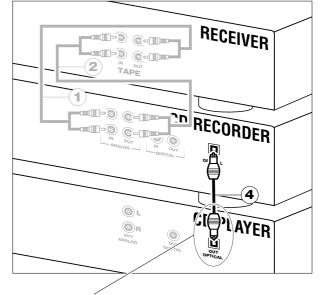
When connecting the Digital Optical cable, make sure it is fully inserted until there is a click.
