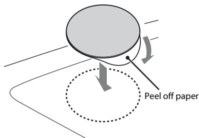
Allow 24 hours after sticking the mounting sheet on the dashboard before installing the cradle on it.
