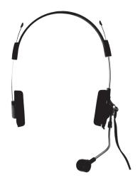
Shure Model 512 combines an efficient "open-air" headphone with a close-talking dynamic microphone. The unit is unobtrusive, durable, comfortable, and provides a wide frequency range.
