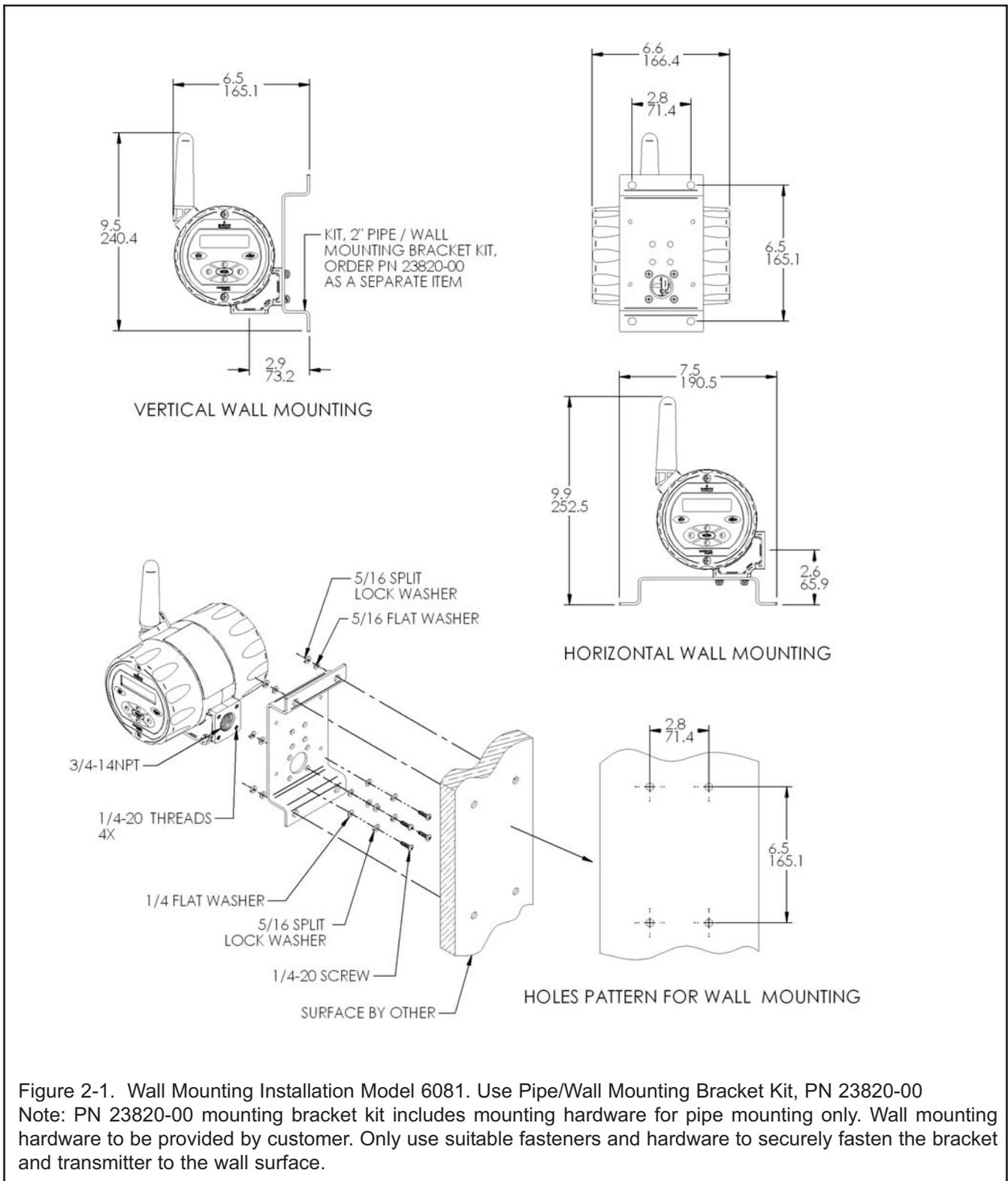
Figure 2-1. Wall Mounting Installation Model 6081. Use Pipe/Wall Mounting Bracket Kit, PN 23820-00
