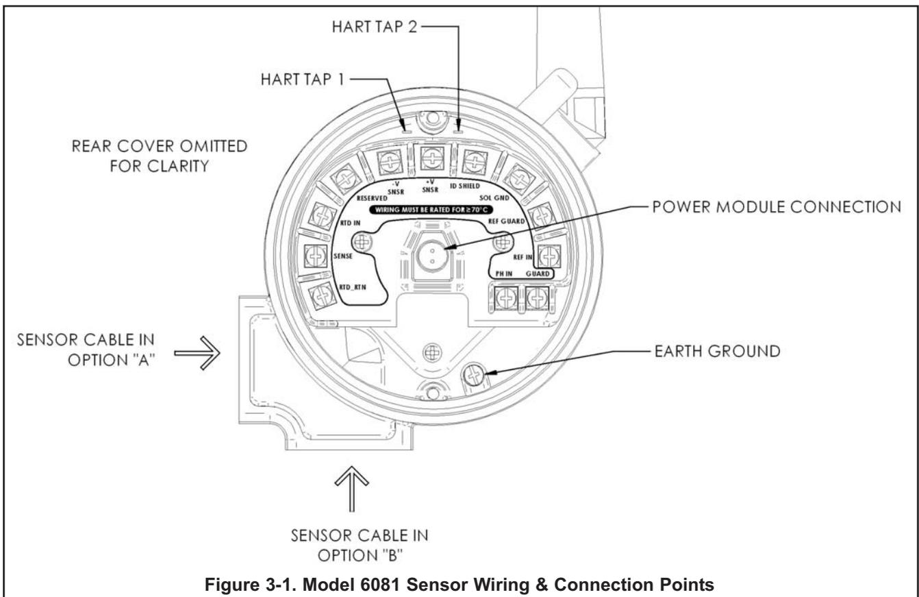
Figure 3-1. Model 6081 Sensor Wiring & Connection Points
