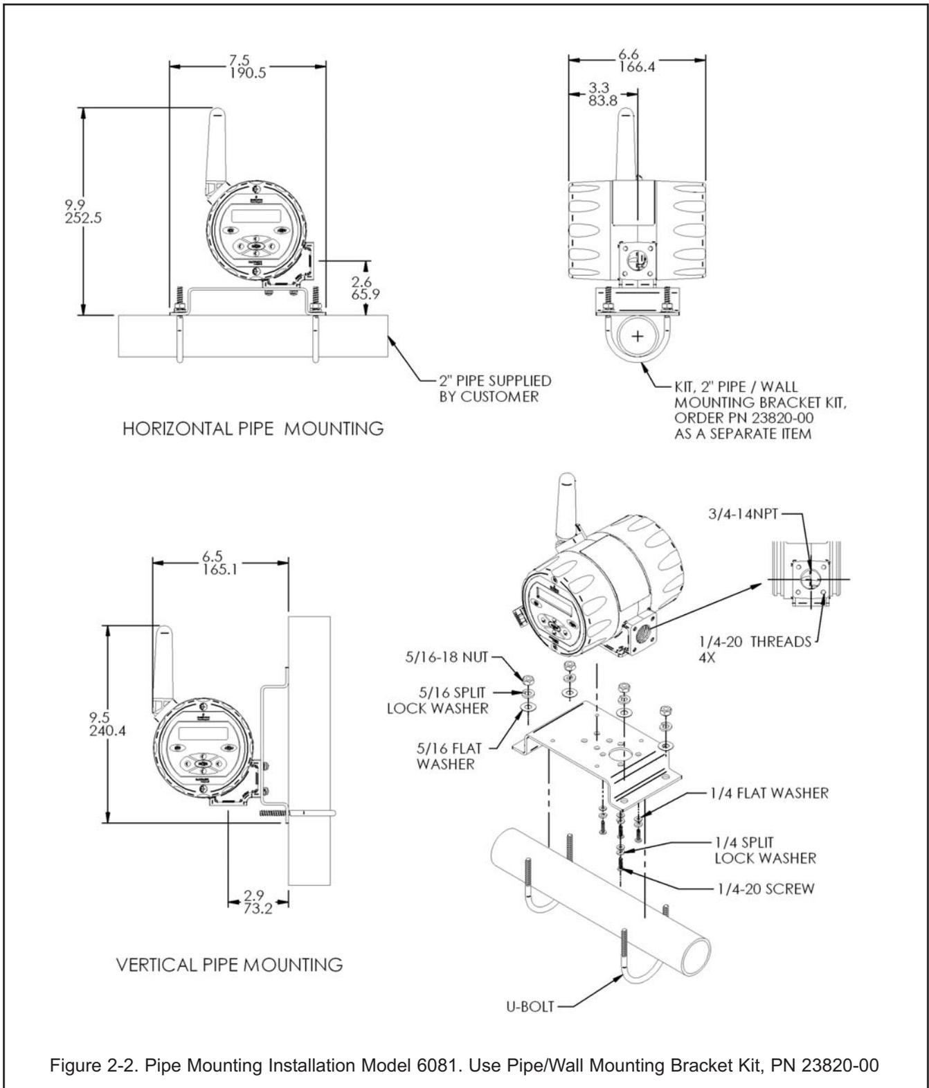
Figure 2-2. Pipe Mounting Installation Model 6081. Use Pipe/Wall Mounting Bracket Kit, PN 23820-00
