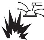
**WELDING SPARKS can cause fire or explosion.**
