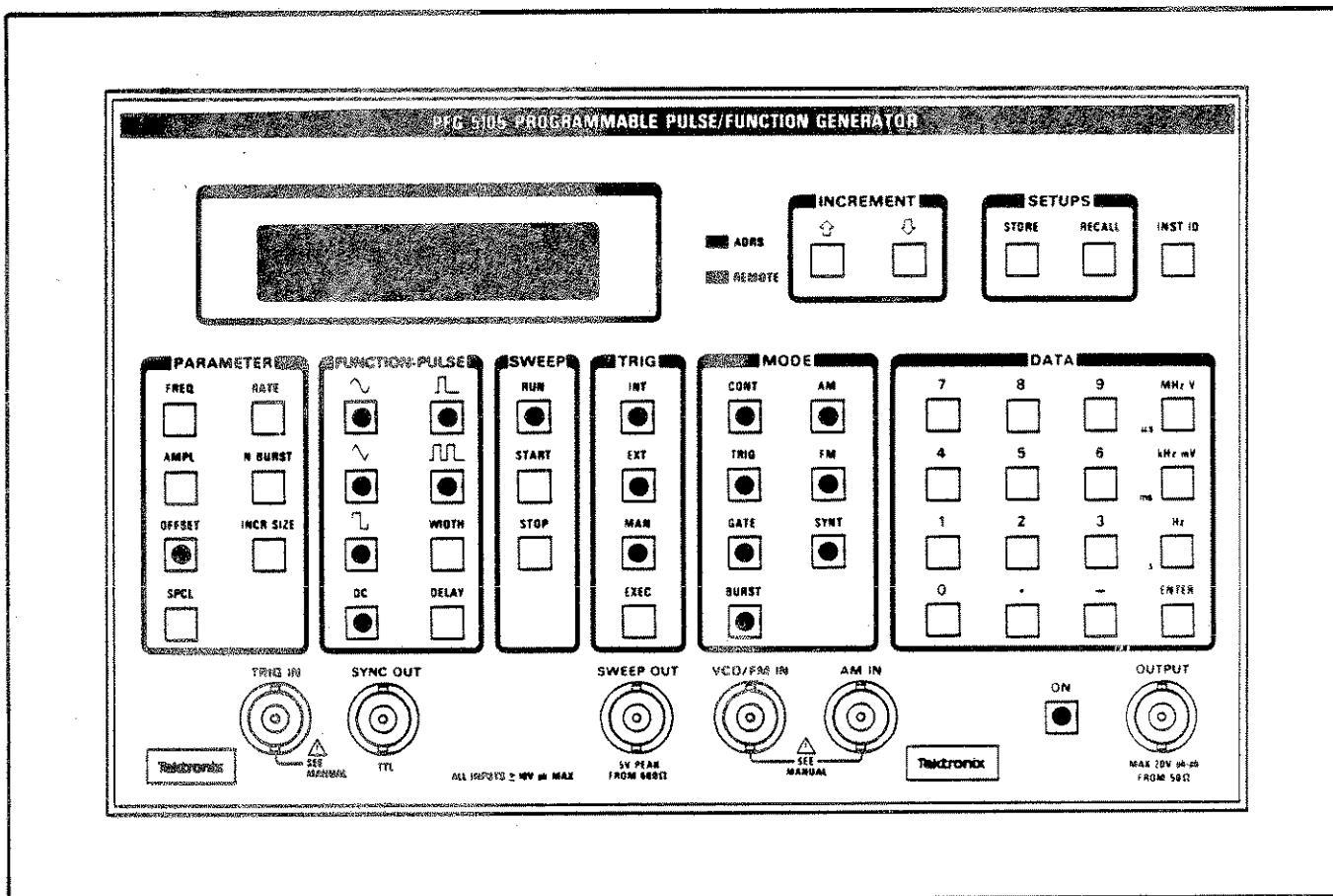
This interfacing guide is designed to help you get started, as quickly and easily as possible, using the PFG 5105/5505 Programmable Function Generator with a GPIB controller. This guide tells you how to program the Tektronix PEP 301 and 4041 controllers to communicate with the PFG 5105/5505. Sample programs are included.
