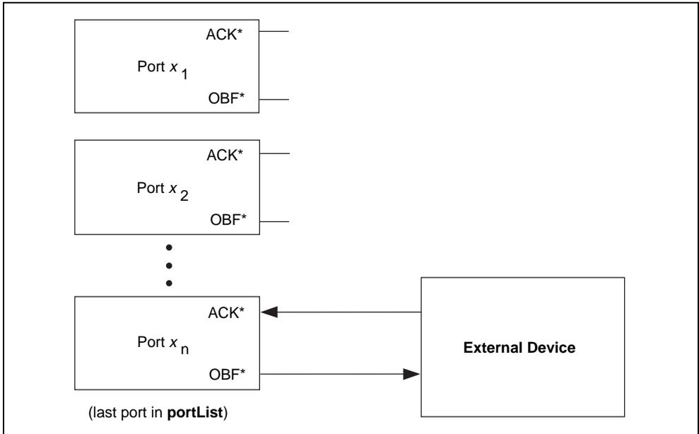
**Figure 2-13.** Digital Scanning Output Group Handshaking Connections
