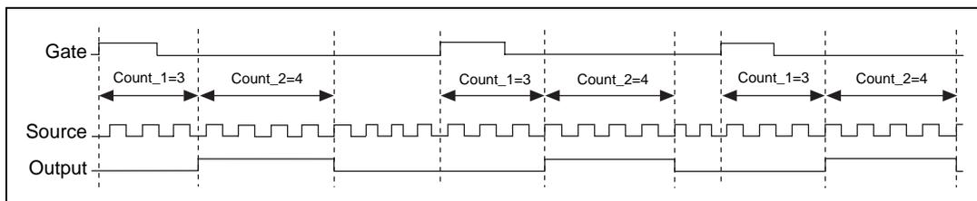
**Figure 2-21.** Retriggerable Pulse Generation
