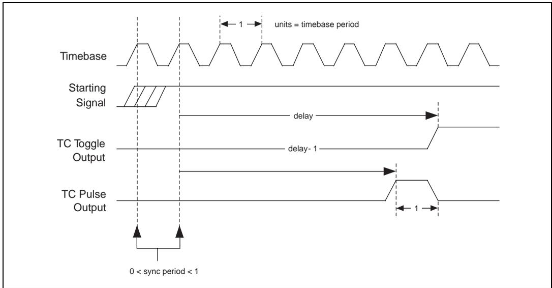
**Figure 2-10.** Pulse Timing for pulseWidth = 0
