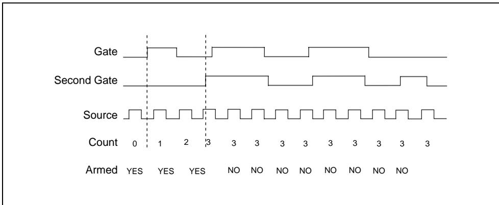
**Figure 2-18.** Start-Stop Measurement
