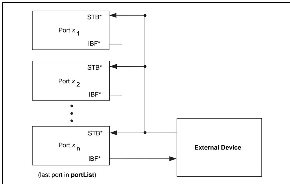
**Figure 2-12.** Digital Scanning Input Group Handshaking Connections
