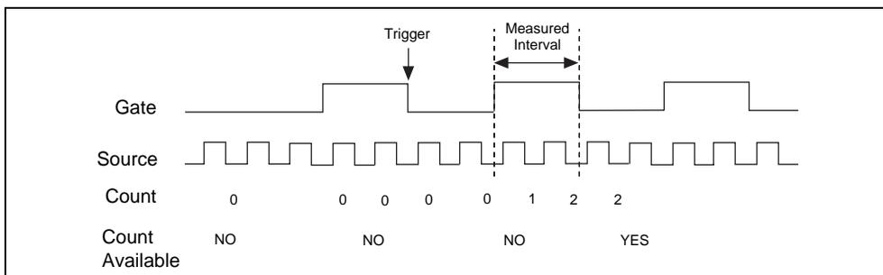
**Figure 2-17.** Single Triggered Pulse Width Generation Measurement
