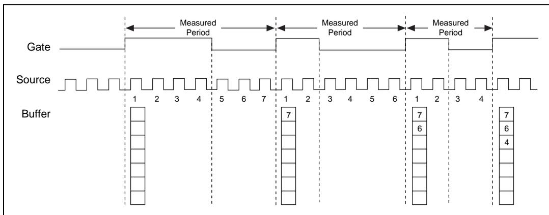
**Figure 2-25.** Buffered Period Measurement
