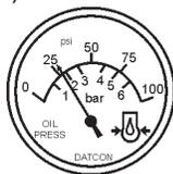
**Figure 46. Oil Pressure Gauge**
