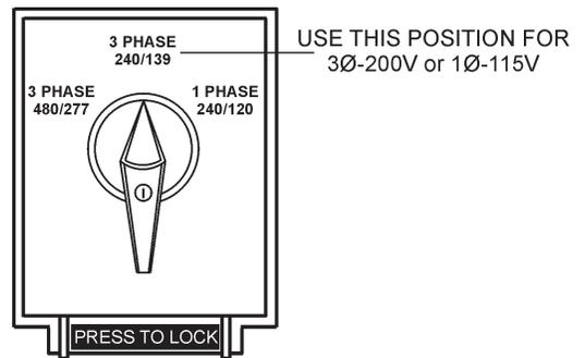
**Figure 21. Voltage Selector Switch
