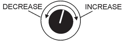
**Figure 20. Voltage Regulator Knob**
