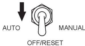
**Figure 54. MPEC Control Switch (Off/Reset)**
