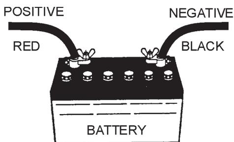
Figure 34. Battery Connections
