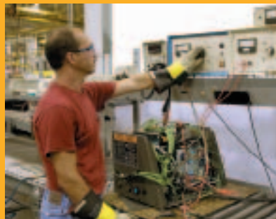
Dielectric tests provide evidence that electrical insulation will withstand the rigors of the welding environment.
