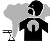
**Fumes and slag generated from Innershield type electrodes recommended for use with this welding machine can be toxic.**
