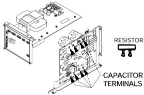
3. Use a DC voltmeter to check that voltage is not present across the terminals on all four capacitors.
