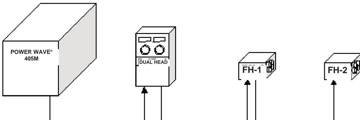
In this case the individual feed heads need to be assigned to the dual head control and the POWER WAVE® 405M auto mapping disabled and the Equipment Groups set on (See Figure A-8). (See the Feeder documentation for information on setting the feeder DIP switches)
