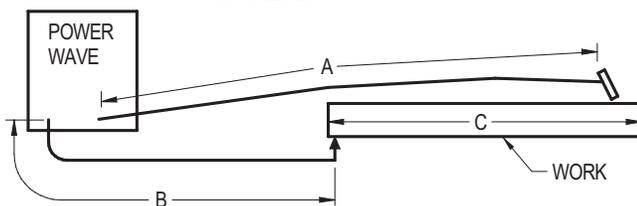
For long work piece lengths, a sliding ground should be considered to keep the total welding loop length less than 50 ft.(15.24m). (See Figure A.4.)
