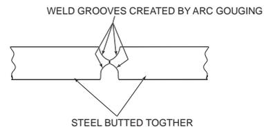
Mode 9 in the POWER WAVE® 405M is specifically for gouging. Gouging can also be done in the stick soft and crisp modes. Setting the output of the Stick Soft mode to 425 amps will enable the arc-gouging mode. The actual output current will depend on the size of carbon used. The recommended maximum size carbon is 5/16".
