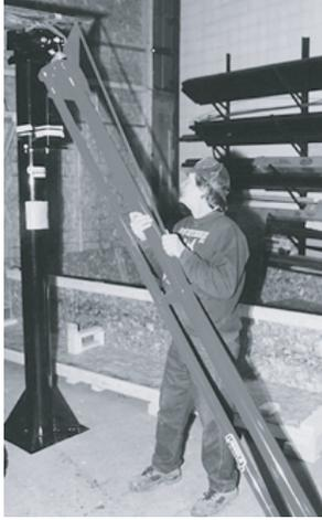
11. Raise the front of the arm with a forklift or hoist and attach to the appropriate hole in the clevis and arm triangle.
