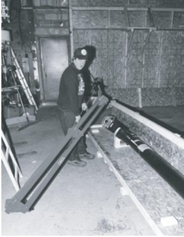
5. Remove the two 3/8" lag bolts from the base of the stanchion. Note: Do NOT remove the steel strap until the stanchion has been secured.
