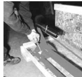
3. Remove the mounting block at the front of the arm.
