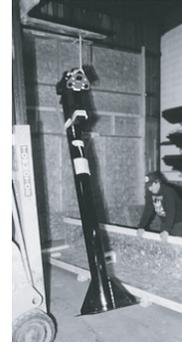
8. Secure the stanchion to the floor per qualified engineer specifications or secure the stanchion to the optional platform. If using the platform, level the platform before installing the stanchion. Install and secure at least 300# of weight onto the platform. A welding power source may be sufficient for this purpose. Verify the weight of the power source.
