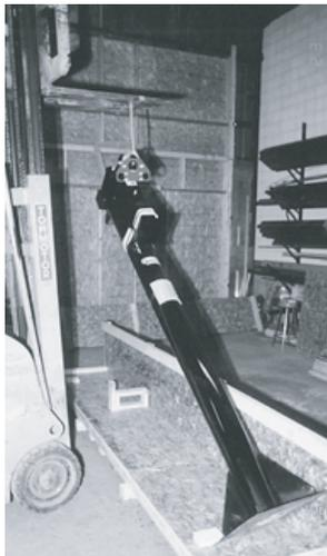
9. Remove the six 1/2" x 1-1/4 bolts and lock washers from the rear of the arm.
