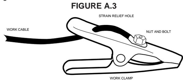
1. Insert the work cable terminal lug with the larger hole through the strain relief hole in the work clamp as shown above.
