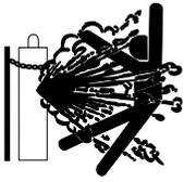
**CYLINDER may explode if damaged. Keep cylinder upright and chained to support**
