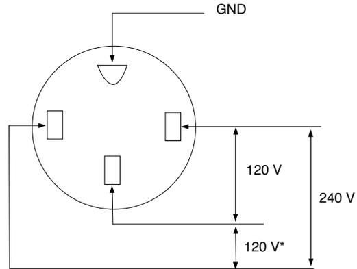
\*Current Sensing for Automatic Idle.
