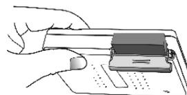
"Insert the battery in accordance with the +/- sign shown on the battery sticker"
