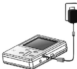
Close the battery cover. Connect one end of the AC Adapter to the DC IN jack of the PVR, the other end to a wall outlet. The red LED will light during battery charging. Charge the battery for at least 3 hours before using for the first time.
