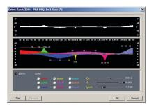
The DriveRack 220i provides both input and output EQ. Input EQ is switchable between a 28-band or 15-band Graphic EQ, or a 9-band Parametric EQ; the output EQ is a 4-band Parametric EQ.
