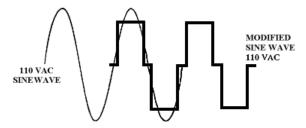
The modified sine wave produced by our inverters has a root mean square (RMS) voltage of 110 volts. The majority of AC voltmeters are calibrated for RMS voltage and assume that the measured waveform will be a pure sine wave.
