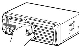
Use the supplied disc magazine or the disc magazine XA-250. The disc magazine XA-10B/XA-350 cannot be used with this unit. If you use any other disc magazine, it may cause a malfunction.
