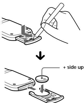
Replace the battery with a Sony CR2025 or Duracell DL-2025 lithium battery. Use of another battery may present a risk of fire or explosion.
