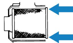
The critical sealing area will stretch slightly, adjust itself and distribute the sealing pressure evenly. To complete a tight seal, apply pressure by hand at the outer rim of the filter, not the flexible center. (Avoid pushing on the center of the urethane end cap.) No cover pressure is required to hold the seal. NEVER use the service cover to push the filter into place! Using the cover to push the filter in could cause damage to the housing, cover fasteners and will void the warranty.
