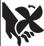
1.f. Do not put your hands near the engine fan. Do not attempt to override the governor or idler by pushing on the throttle control rods while the engine is running.
