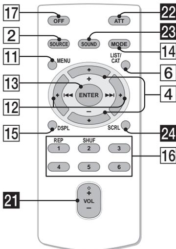
Refer to the pages listed for details. The corresponding buttons on the card remote commander control the same functions as those on the unit.
