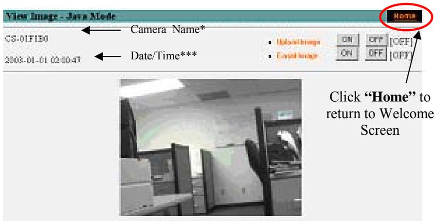
**Camera Name\*** - The Camera name will be display when the Camera Name field is entered in the Web Configuration setting under “**System**”
