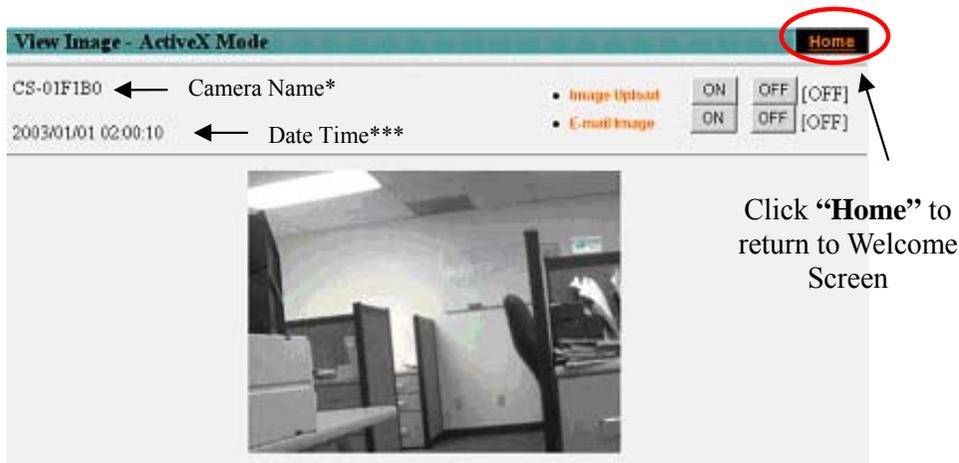
**Camera Name\*** - The Camera name will be displayed when the Camera Name field is entered in the Web Configuration setting under **“System”**
