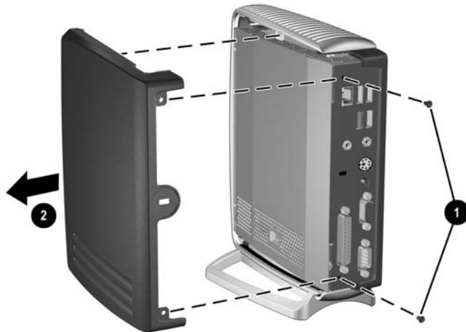
Removing the Side Access Panel
