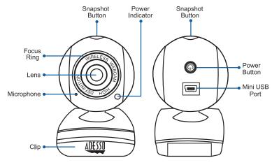
**NOTE:** To adjust focus use the Focus Ring located in front of lens.
